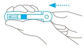
Make sure you position the blade **exactly over the locating lugs**, close the blade holder upwards. **Attention:** Never hold your hand in front of the blade exit!
