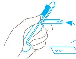
Use your index finger to slowly **fold out the blade holder downwards**. Use the other hand to remove the blade to either replace it or turn it around (for left handers).
