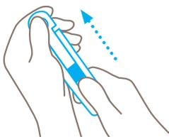
Use the slider to **push** the plastic insert back and out of the handle. **Don't** pull the insert while holding onto the slider.
