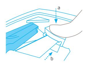
In order to insert a **new blade** press the centre of the blade holder again (a). At once push the blade into the blade holder until the **hole** formation can no longer be seen (b).
