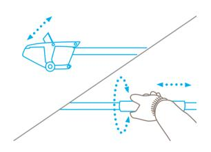
After successfully changing the blade, please check whether the **release and retraction** of the blade is functioning properly.
