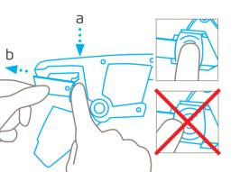
Now push the **centre** (a) of the blade holder (within the crosshatched area) and remove the blade with the other hand **simultaneously** (b).
