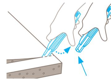
Following cutting, the blade immediately retracts into the handle. **CAUTION: Don't block the slider** with your hand.
