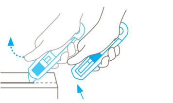
Following cutting, the blade immediately retracts into the handle. Condition: you have released hold of the slider.
